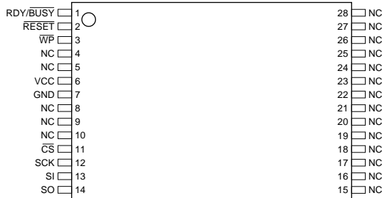
TSOP Top View – Type 1
