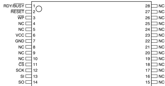
Figure 2-2. CASON – Top View through Package
