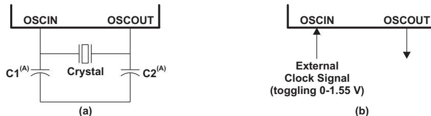
Figure 5-3. Recommended Crystal/Clock Connection
