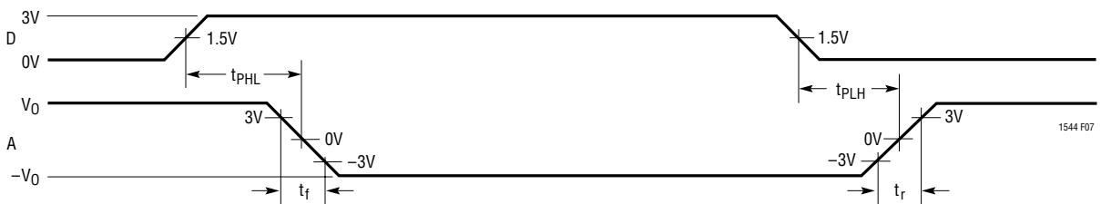
Figure 7. V.10, V.28 Driver Propagation Delays
