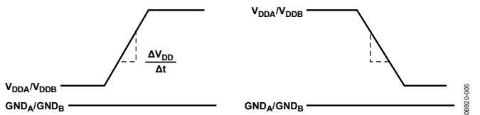
Figure 14. Transient Immunity Waveforms, Output Supplies
