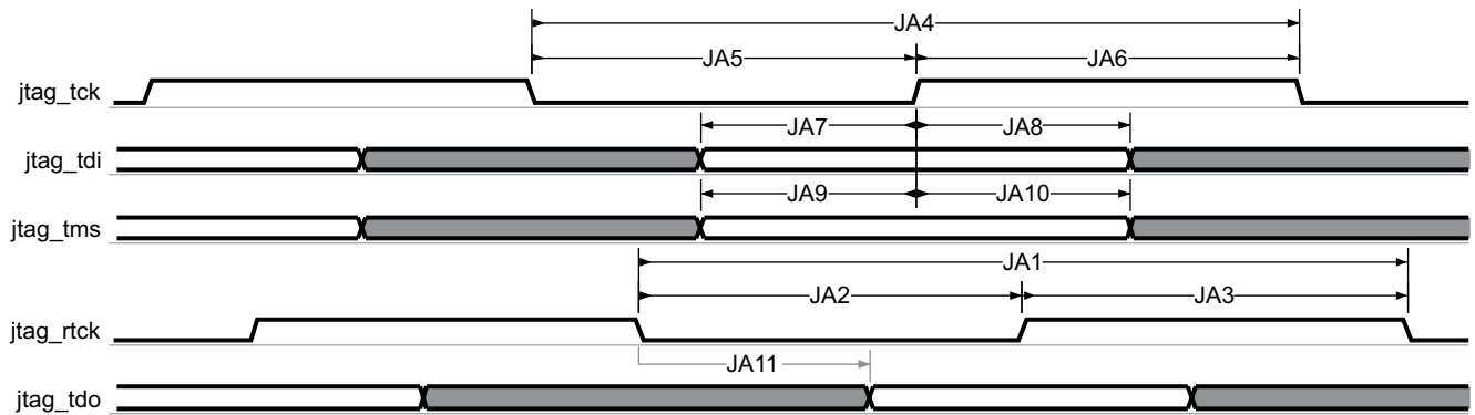
Figure 6-83. JTAG—Adaptative Clock Mode
