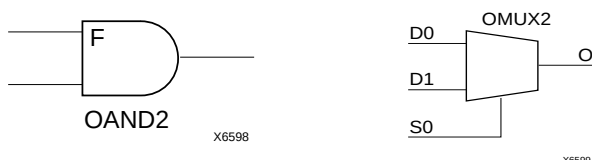
Figure 20: AND & MUX Symbols in XC4000X IOB
