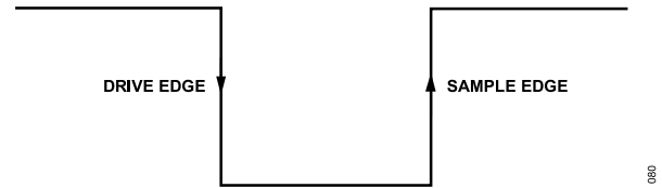
Figure 78. SPI Mode 0 SCLK Edges
