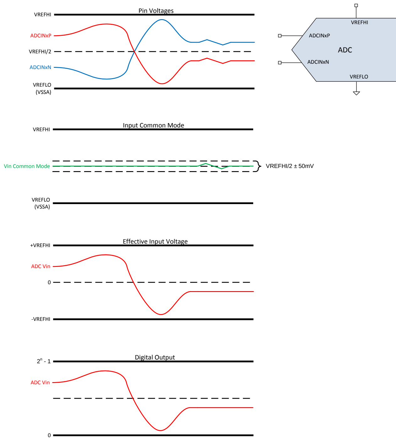
Figure 5-31. Differential Signaling Mode
