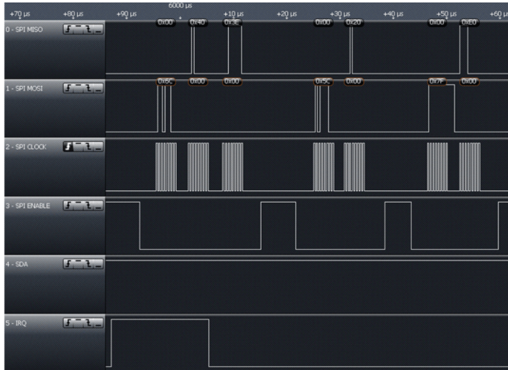
Figure 6-24. IRQ With One Byte in FIFO
