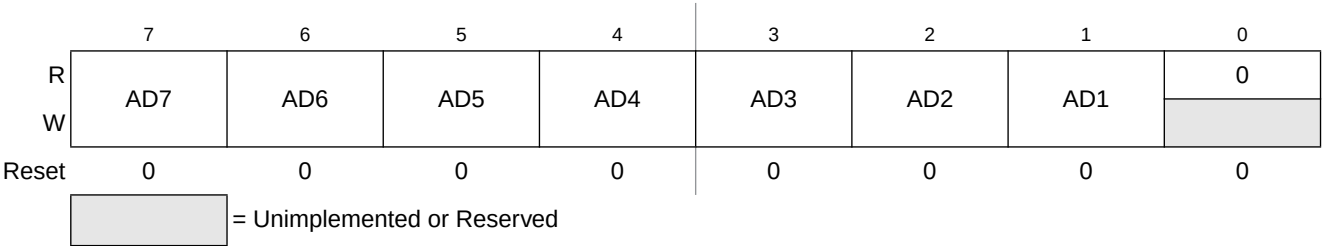
Figure 11-3. IIC Address Register (IICxA)
