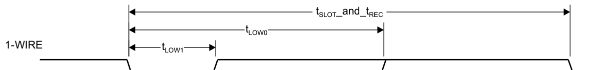
Figure 5-118. 1-Wire Write Bit Timing (Command/Address or Data)
