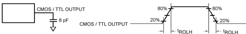
Figure 9. Receiver LVTTTL/CMOS Output Load and Transition Times
