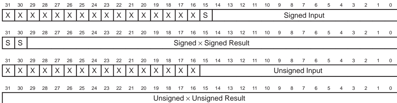
Figure 39. 16 x 16 Multiplier Data Formats
