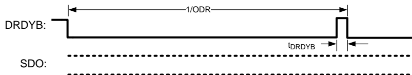
Figure 62. DRDYB Behavior for an ADC_DOUT not Read
