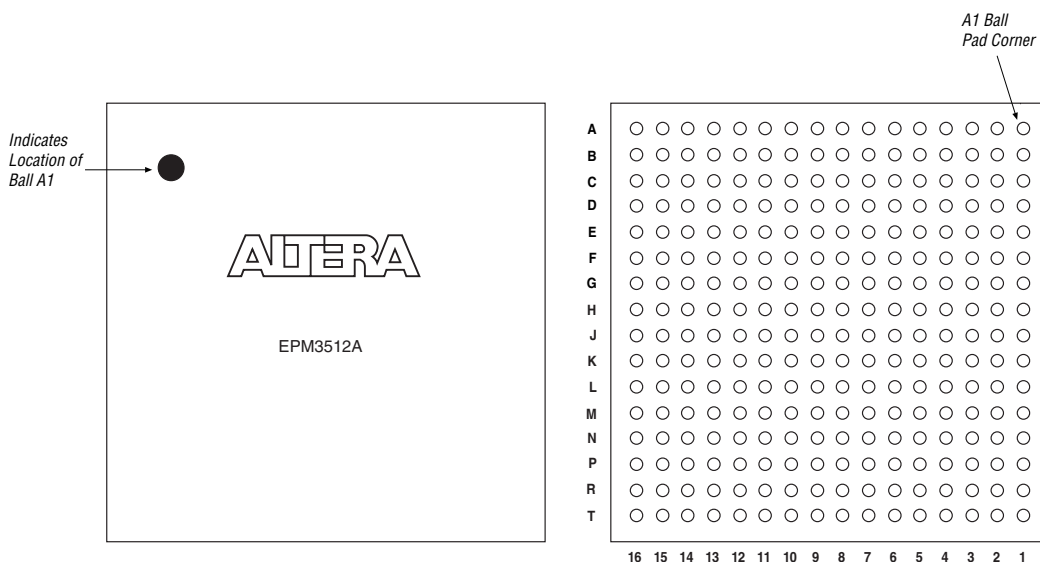
Figure 18. 256-Pin FineLine BGA Package Pin-Out Diagram
