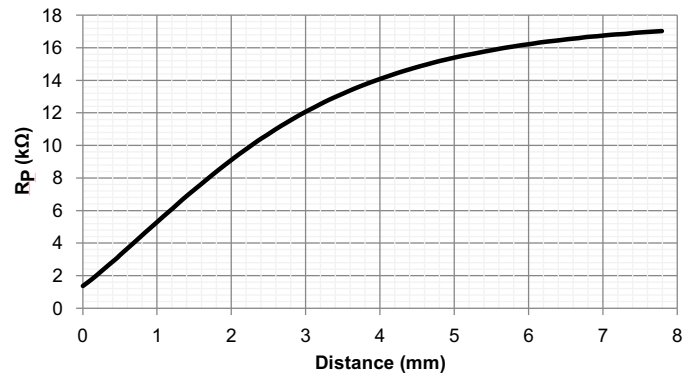
Figure 47. Example R_p vs. Distance with a 14 mm PCB Coil and 2 mm Thick Stainless Steel Target
