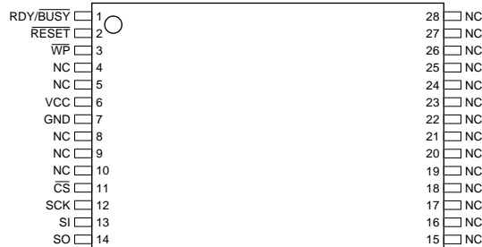
TSOP Top View – Type 1
