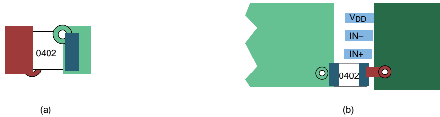
Figure 48. Typical Decoupling Capacitor Layouts
