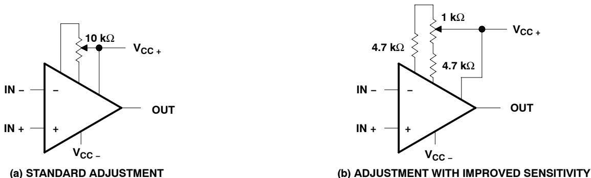
Figure 55. Input Offset Voltage Nulling Circuits
