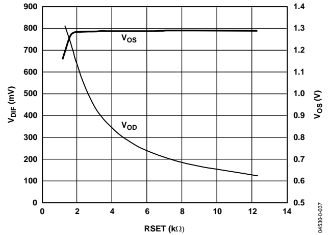
Figure 38. LVDS Output Swing, Common-Mode Voltage vs. RSET, Placed at LVDSBIAS (Both Speed Grades)
