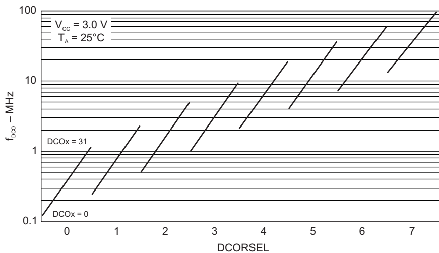
Figure 5-10. Typical DCO Frequency
