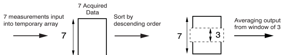
Figure 29. MAV Filter Operation (Patent Pending)
