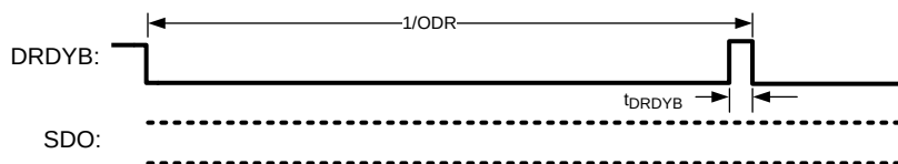
Figure 62. DRDYB Behavior for an ADC_DOUT not Read
