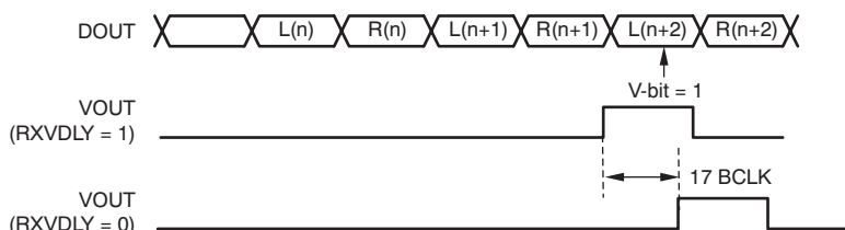
Figure 26. RXVDLY and VOUT Timing
