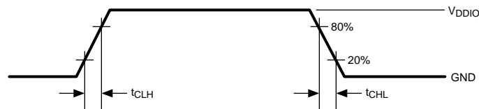
Figure 10. Deserializer LVCMOS Transition Times
