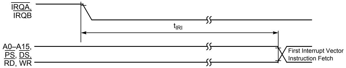
Figure 3-17 Interrupt from Wait State Timing
