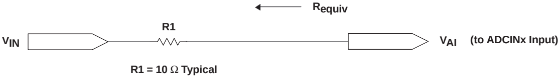
Figure 41. Typical ADC Input Pin Circuit
