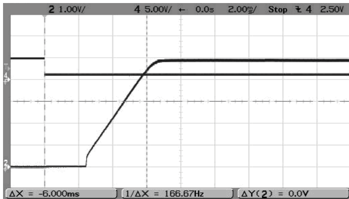
On/Off Enable Startup Delay (Vin=12V, Vout=5.0V, Iout=3A, Clad=0) Trace 4=Enable In, Trace2=Vout
