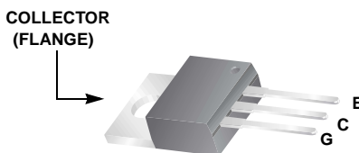
JEDEC TO-220AB ALTERNATE VERSION
