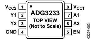
Figure 6. 8-Lead MSOP Package (RM-8)
