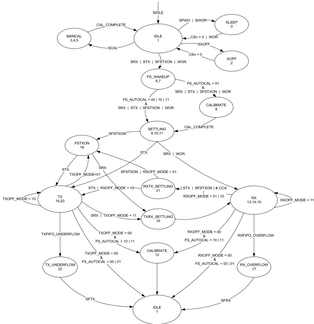
Figure 25: Complete Radio Control State Diagram
