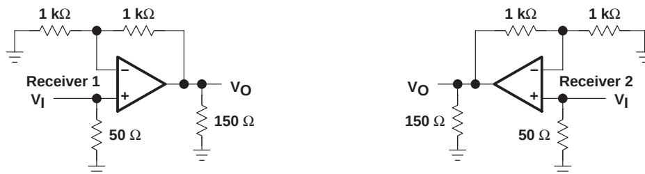
Figure 2. Receiver Input-to-Output Crosstalk Test Circuit
