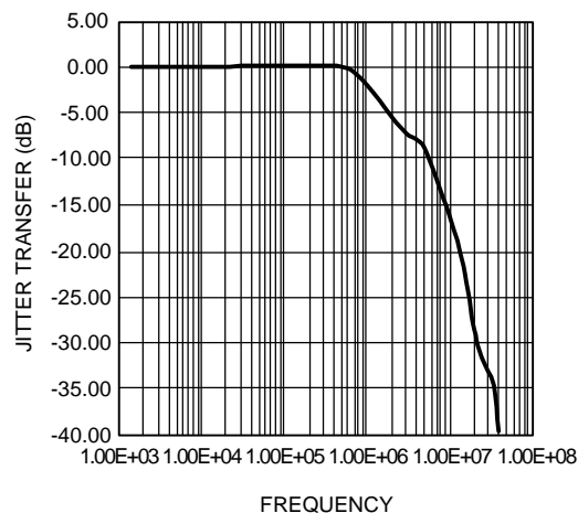
Figure 10. Jitter Transfer Curve
