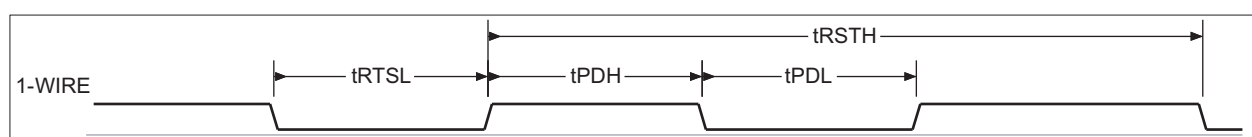
Figure 6-61. 1-Wire Break (Reset) Timing
