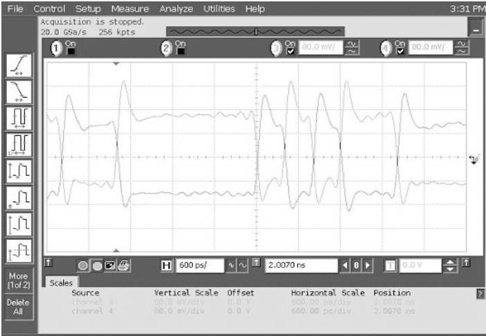
Data Waveforms, 2.5Gbps (left) & 5.0Gbps (right)
