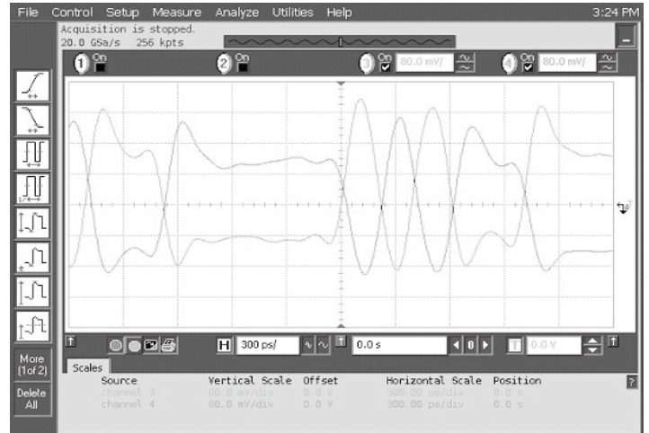
Data Waveforms, 2.5Gbps (left) & 5.0Gbps (right)
