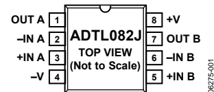
Figure 1. 8-Lead SOIC_N (R-8)
