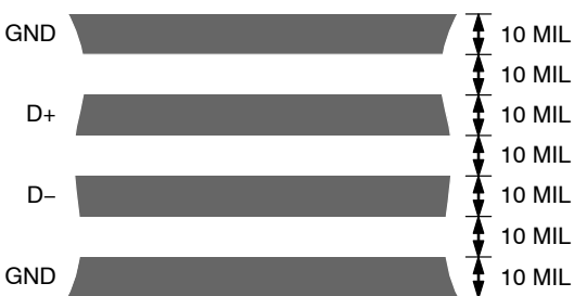
Figure 18. Typical Arrangement of Signal Tracks
