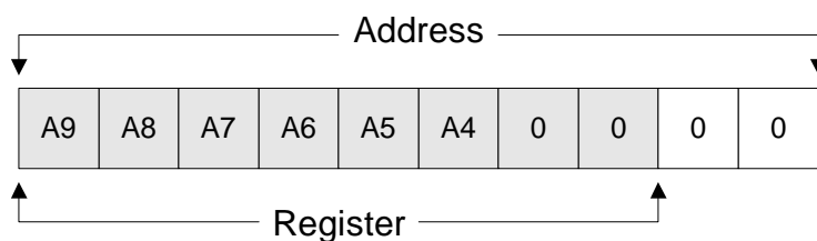
Figure 8-4. FIFO Start Address Format
