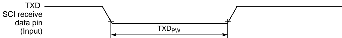
Figure 3-26 TXD Pulse Width
