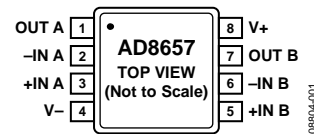
Figure 1. AD8657 Pin Configuration, 8-Lead MSOP
