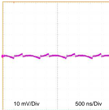
12\text{ V}_{IN} 3.3\text{ V}_O at 5\text{ A} , \text{BW} = 20\text{ MHz}
