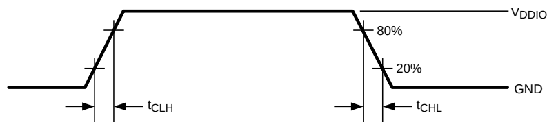
Figure 10. Deserializer LVCMOS Transition Times
