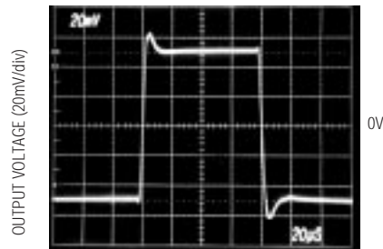
TIME (20 \mu s/div) A_V = +1, C_L = 15pF
