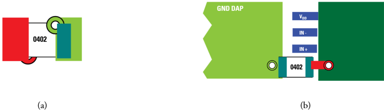
Figure 30. Typical Decoupling Capacitor Layouts
