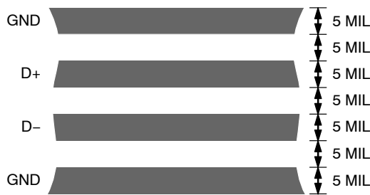
Figure 21. Typical Arrangement of Signal Tracks
