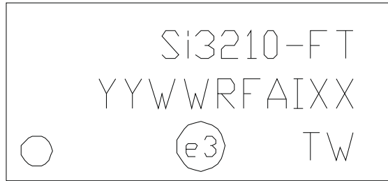
Figure 40. TSSOP Top Mark Diagram
