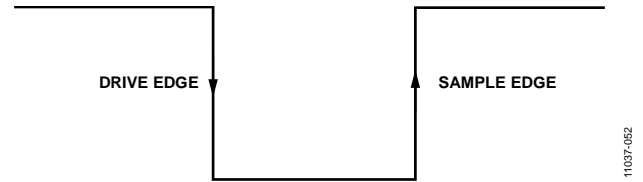
Figure 38. SPI Mode 3 SCLK Edges
