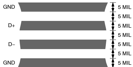
Figure 16. Arrangement of Signal Tracks
