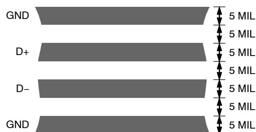
Figure 16. Arrangement of Signal Tracks
